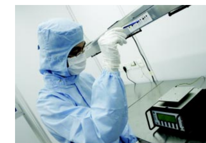
Figure 4: Calibration / Adjustment of Ionizer
