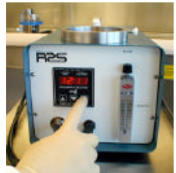
9) When the test period is complete, stop the sample cycle, or the sample cycle will self terminate at the end of the pre-set test period interval.
