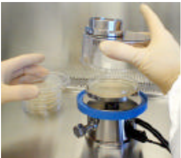
10) Remove the dome assembly and replace the test plate lid.
