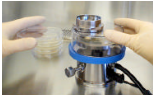
4) Replace the dome assembly and ensure that the dome is properly seated in the seal. Place the test plate lid next to the sampler on a sanitized surface.
