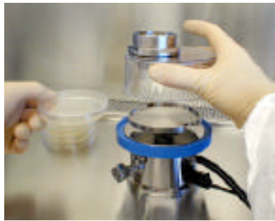
2) Remove the dome assembly, retaining it over the sampler to minimize the risk of incidental contamination.
