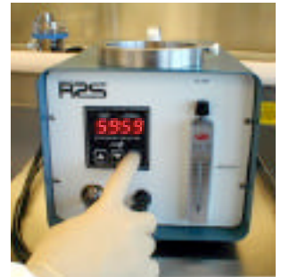
6) Set the desired test period interval (from 1" to 59'59") and start the sample cycle.
