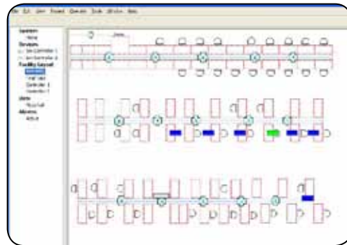
The facility layout view provides mouse-over status reporting with click and drag and click ionizer layout capability.
